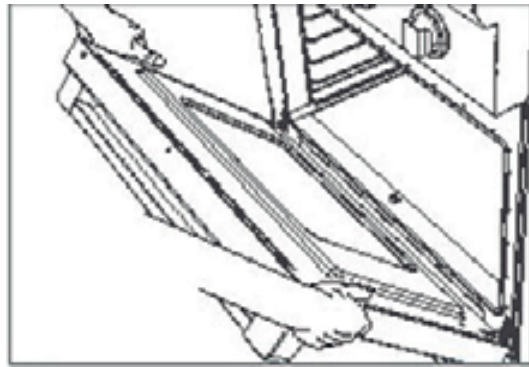
4. Disengage the hinges and remove the door, place on a protected surface.
