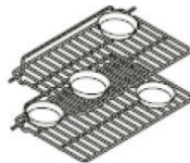
Multiple rack pan placement
