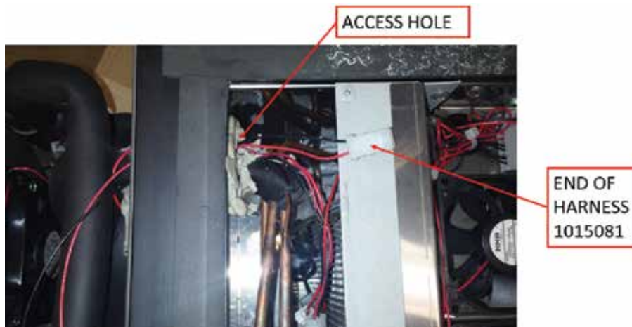
Figure 6-15.8. Feed Harness End Through Access Hole
