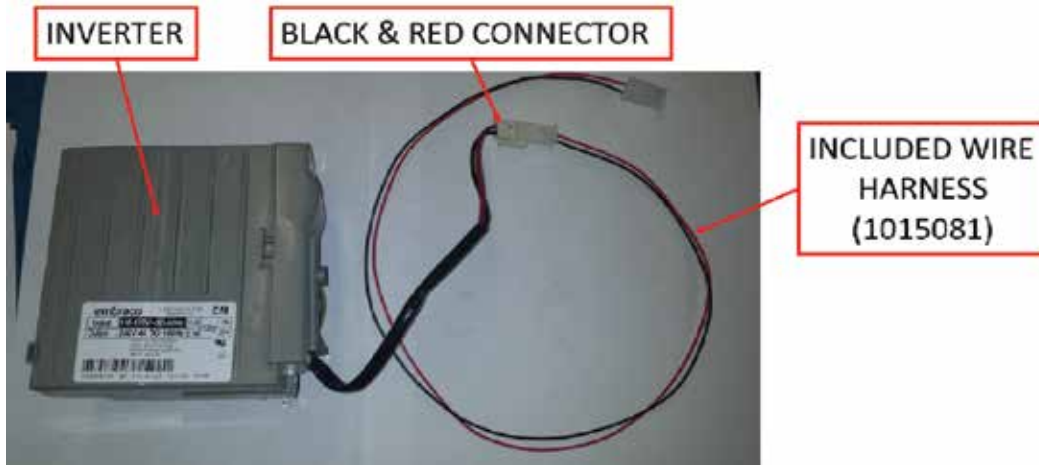
Figure 6-15.7. Connect Inverter Wires
