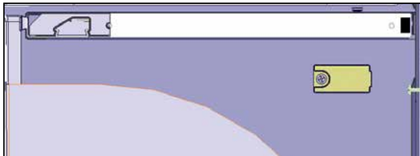
Figure 7-3.7. Refrigerator Tip-Out Bin Temp/Humidity Sensor
