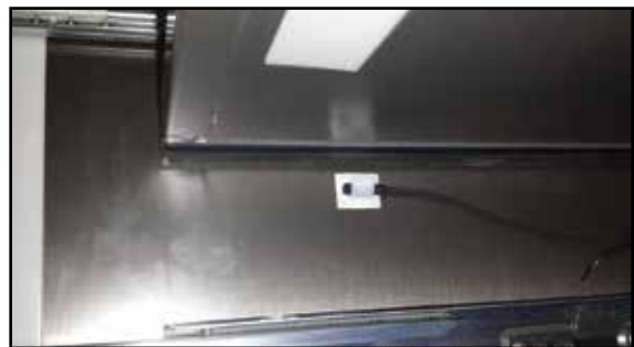
Figure 7-3.6. Refrigerator Meat/Fish Bin Temperature Probe
