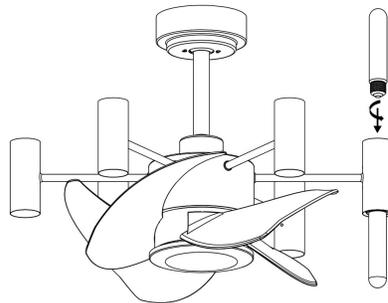
Holding gently the lamp arm, take a glass shade and install it over the bulb turning it clockwise. Tighten. Install the other 11 glass shades.
