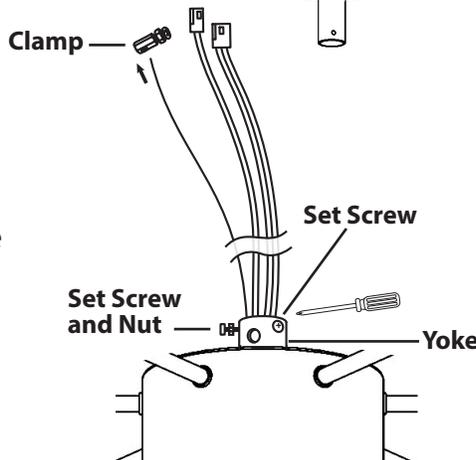
4. Thread the wires and safety cable that comes from the Motor assembly through the Down Rod.
