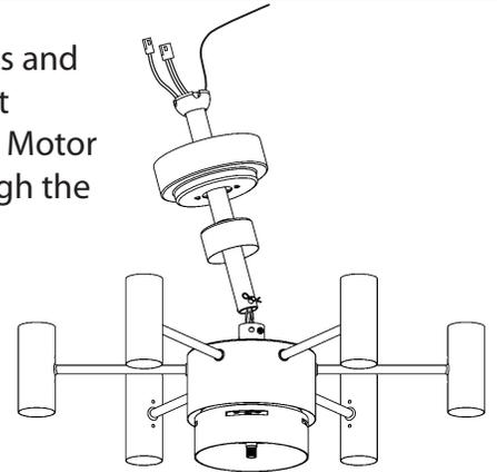
5. Insert the Down Rod into the Yoke making sure that the wires are not twisted and aligning the holes for the pin on the Down Rod with the holes in the motor Yoke. Insert Pin all the way through and put the Clip in place. Secure tightly the 2 Set Screws and Nut. Lower Yoke Cover until it rests on the Motor Assembly.
