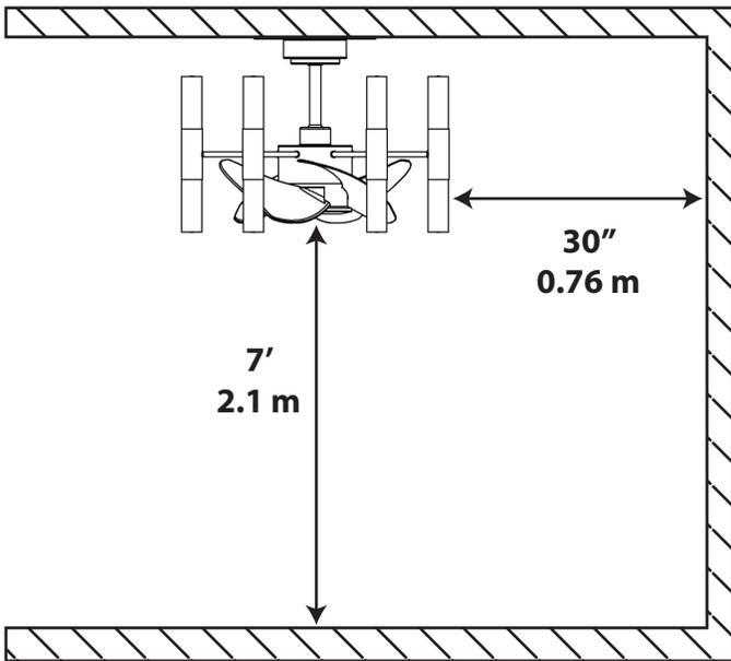
This fan can be mounted with the down rod (5) in a flat ceiling or a vaulted ceiling as long as the angle of the ceiling is under 19 degrees.
