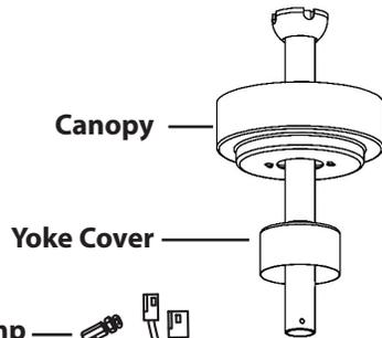
3. Loosen the Set Screw and Nut and the Set Screw on the Yoke. Take the Clamp out from the Safety Cable.
