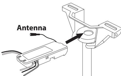
Gently insert the receiver into the Mounting Bracket with the flat part towards the top. Carefully push wires and wire connectors into the electric box leaving the antenna outside of the Mounting Bracket.
