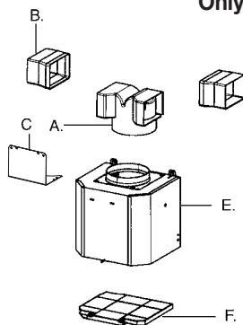
Ductless installations require a **Ductless Conversion Kit** whose components are pictured in **FIGURE**. Do not use the DAMPER for ductless installations.
