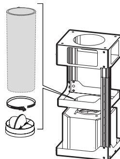
Install Damper that is included with the Hood before connecting to the ductwork.
