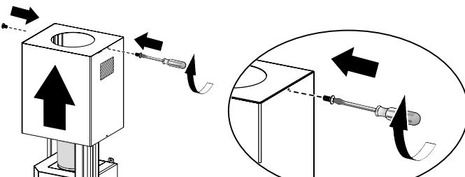
Position the upper chimney section and fix the upper part to the frame using the 2 screws removed previously.
