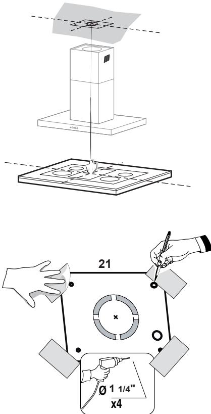
Put a thick, protective covering over cooktop, set-in range or countertop to protect from damage or dirt.
