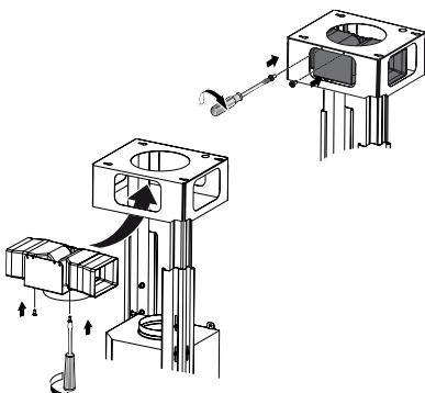
Insert the Connector extensions **B** into the side of the Connector **A**.
