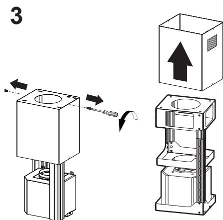
Loosen the two screws fastening the upper chimney and remove this from the upper frame.
