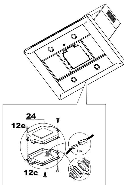
Connect the control connector Cmd and .
