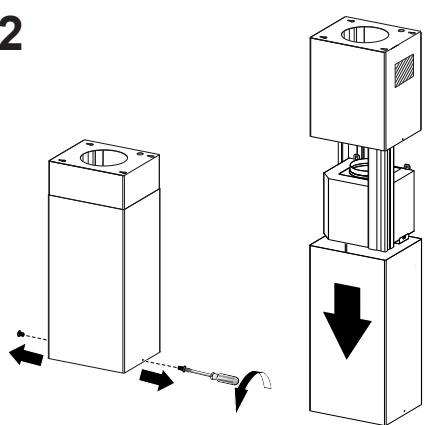
Loosen the two screws fastening the lower chimney and remove this from the lower frame.
