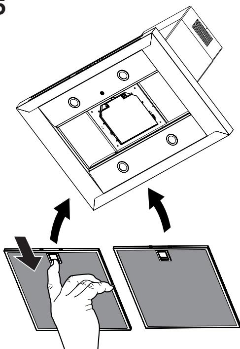
Reinstall the grease filters from the hood canopy.
