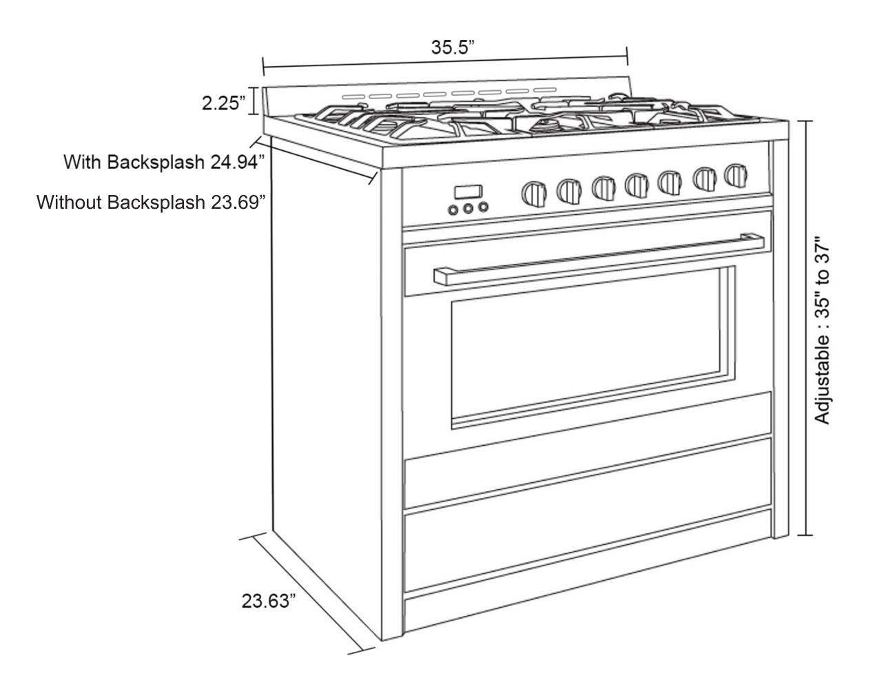
Dimensions (WxDxH): 35.5" x 23.6-25" x 35-37" Overall Interior Oven Dimensions (WxDxH): 26.5" x 18" x 14" Usable Interior Oven Dimensions (WxDxH): 26.5" x 16.75" x 11.5"
