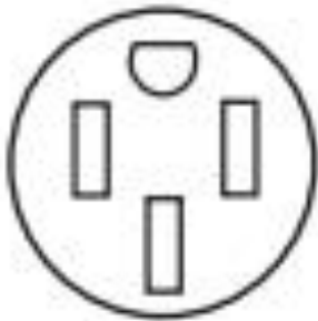
4-wire receptacle (14-50R)
