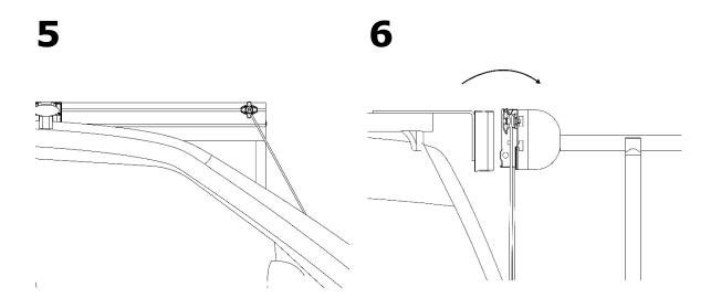
Attach a **pair** of guy ropes to the Prop Cleats at each end of the awning and peg one leg of each **pair** of guys ropes parallel to the vehicle (one to the front and one to the back of the vehicle).
