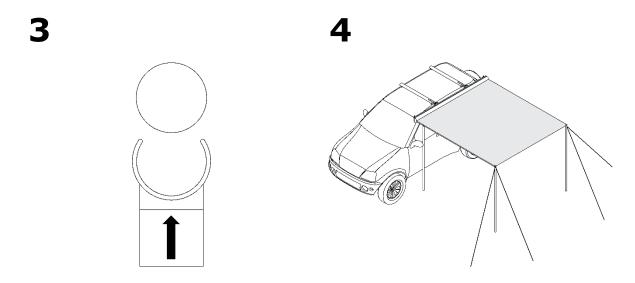
Attach C-clip poles to each horizontal "rafter" bar on the awning, then slide them up towards the vehicle adjusting them for length.
