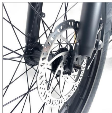
2. Align the front fork with the hub.
