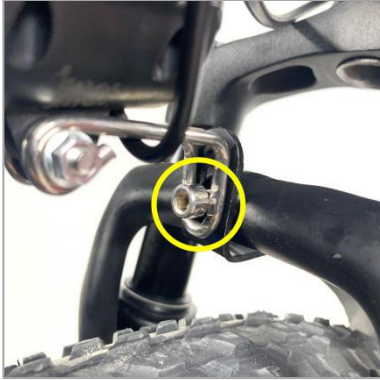
1. The screw for headlight & fender.
