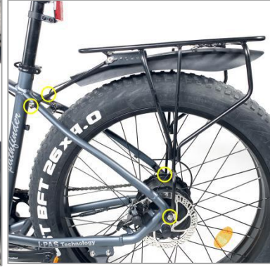
2. Tighten four screws to assemble the rear rack.
