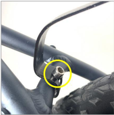
3. Tighten two screws to assemble the rear fender.
