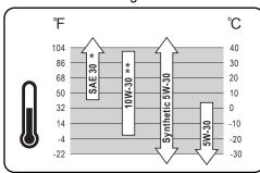
Note: \*Below 40°F (4°C) the use of SAE 30 will result in hard starting. \*\*Above 80°F (27°C) the use of 10W-30 may cause increased oil consumption. Check oil level more frequently
