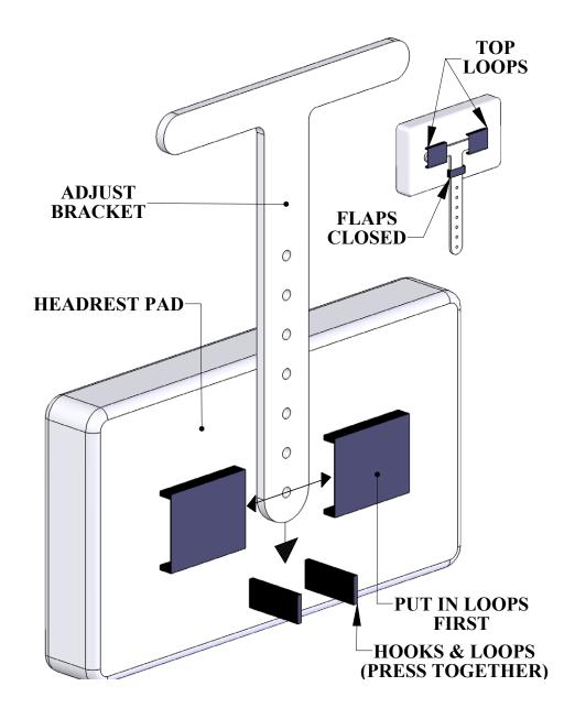
The ADJUST BRACKET must be removed from the assembly to install or remove the HEADREST PAD. When installing the pad thread the bracket through the middle loop first and slide the pad up to the top loops. Thread the bracket through the top loops (one at a time) to complete the installation. To remove the pad, reverse this procedure.
