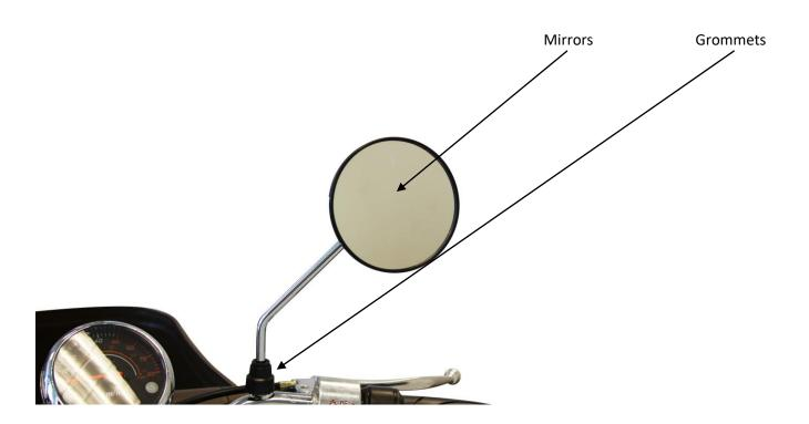
To attach the mirror simply place each mirror threaded end into the mirror post. Turn mirror clockwise and fasten mirror to scooter.
