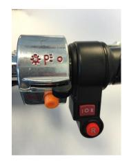
The parking / emergency brake is located on the left-hand brake. The tab holds tension in the brake lines to keep the unit stationary while not in use. Activate by depressing towards the brake handle, while squeezing the brake handle. The tab will click inwards and active once the brake handle is pulled approximately half way. Squeeze the brake handle to deactivate.
