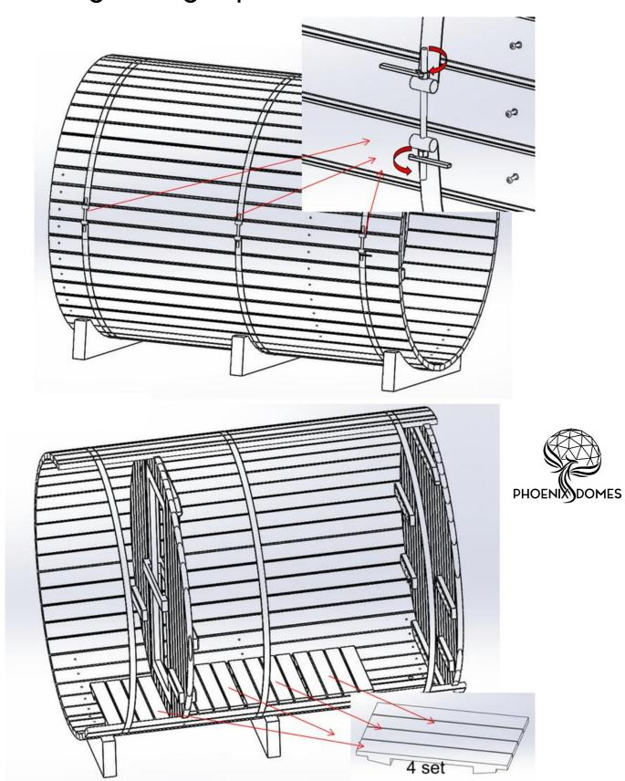
14. Lay down the 4 floor panels as shown
