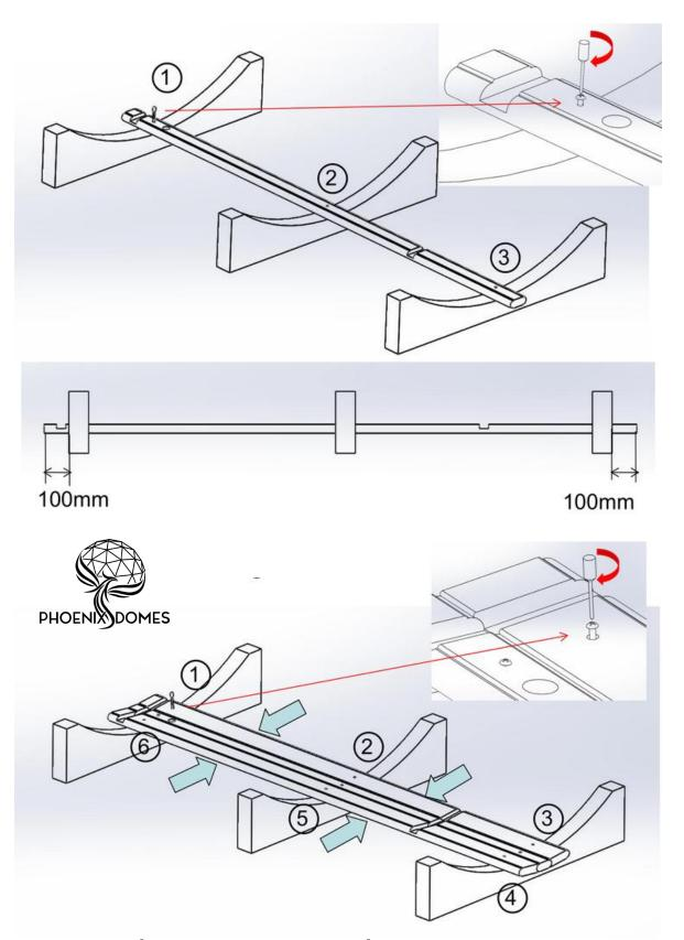
6. Screw in the next two adjacent staves, ensuring the front and back notches are arranged as shown
