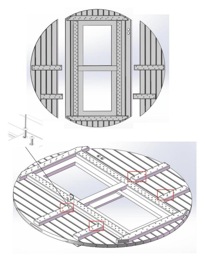
Lay the 3 indicated sections of your sauna's front wall, smooth side down, on a nonmarking surface, and screw them together at the positions indicated
