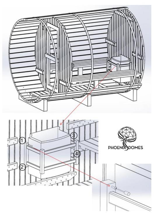
19. Secure your stove to the back wall using its specific hardware and instructions. It will be necessary to drill a hole through the back wall for the power cord - we recommend drilling 2 larger or 3 smaller holes in a row a few inches under the base of the heater in order to provide a small amount of fresh air that will be immediately warmed upon entering your sauna
