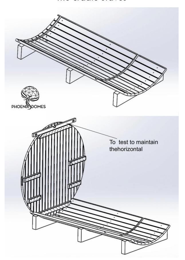
8. Fit your back wall into the back notch, test your level once more, and adjust as necessary
