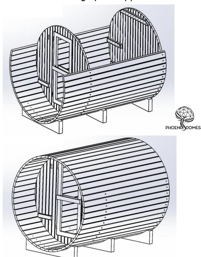
12. Complete the circle, using a rubber mallet to knock any staves into place that resist coming into circular
