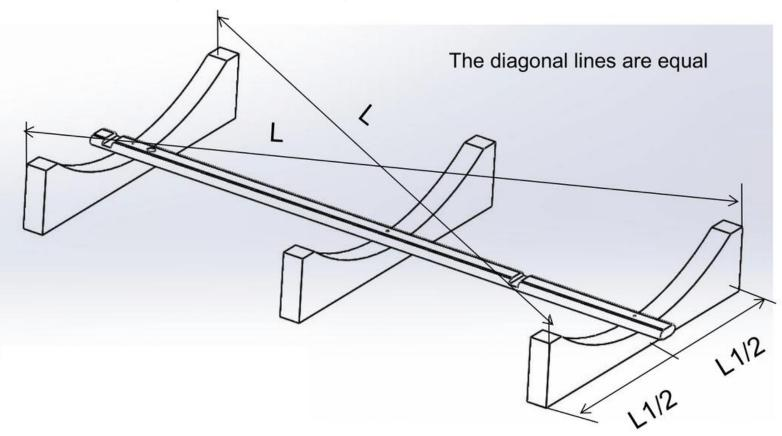
4. Lay down your middle stave (two rounded edges) and test the vertical and diagonal axes
