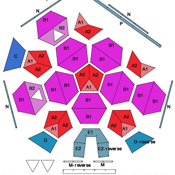
Please note that you can select 2 out of 3 possible positions for the triangle windows and install the insulation accordingly.
