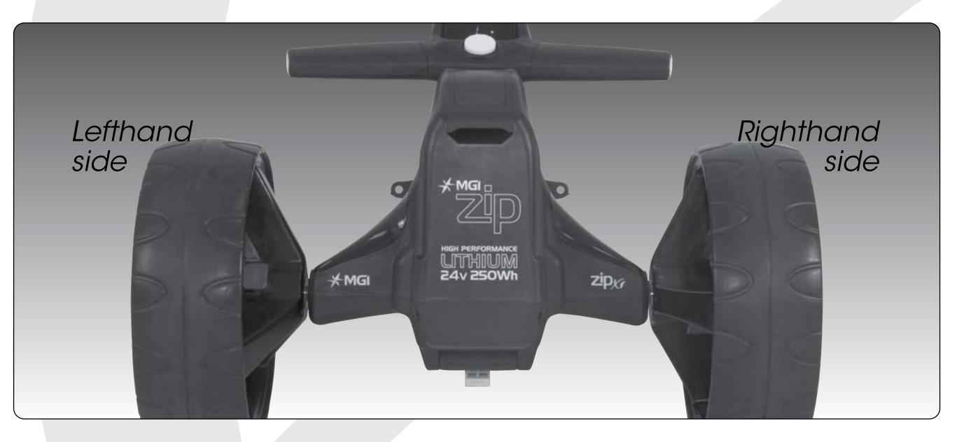
**Step 1.** Each wheel is labelled with L or R for left or right. This is very important as the wheels must be placed on the correct side of the Zip X1. Left or right sides are determined when standing behind the Zip X1 as pictured above.
