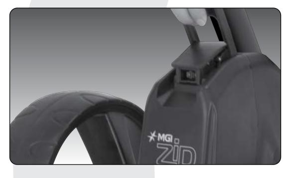
**Step 1:** Disconnect the battery by lifting the battery handle. It can be left on or removed from the Zip X1.
