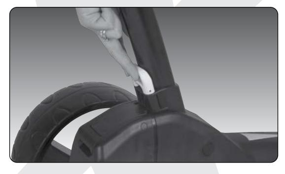
**Step 3:** Pull up the latch at the bottom of the handle.
