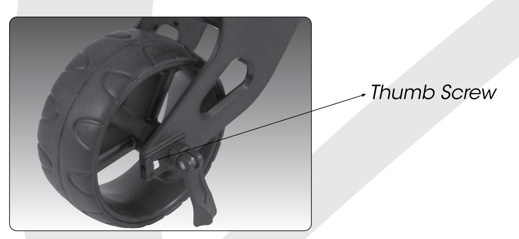
Roll the left or right hand side silver thumb screw UP to straighten the Zip X1 more to the LEFT.
