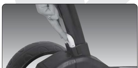
**Step 3:** Pull up the latch at the bottom of the handle.
