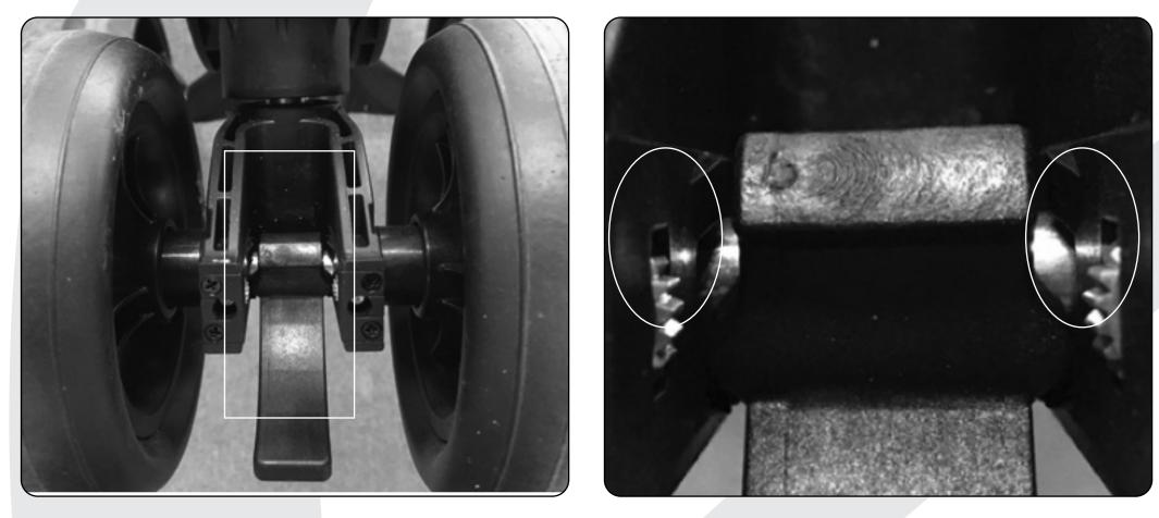
Please note that there is a process in adjusting the tracking. It is suggested that the users should do a little bit of adjustment, test the tracking and then adjust again until the Zip X5 goes straight.
