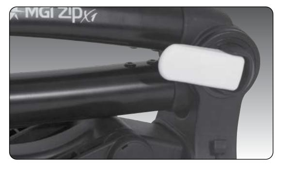
**Step 6:** Close the fold lever to lock the handle into place.
