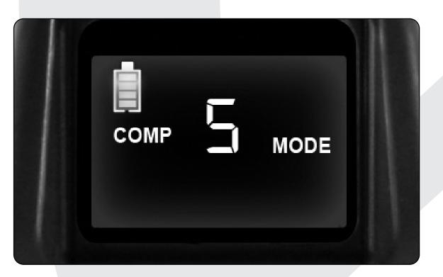
To exit COMP MODE hold down the left and right buttons at the same time.
