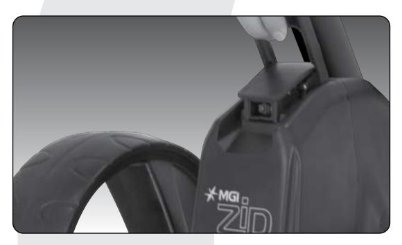
**Step 1:** Disconnect the battery by lifting the battery handle. It can be left on or removed from the Zip X5.
