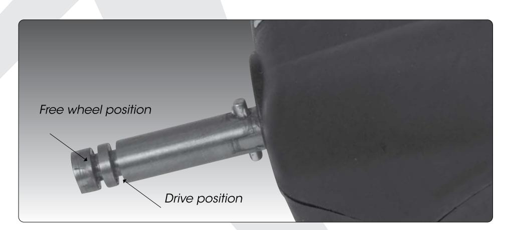
i. Drive position – Lock the wheel onto the groove closest to the battery base. To do this, press the grey release button on the wheel hub, push the wheel on to the axle as far as possible. To test for drive position try rolling the wheel backwards. If you feel resistance then the wheel is now in drive position and ready to use. Repeat for other wheel.
