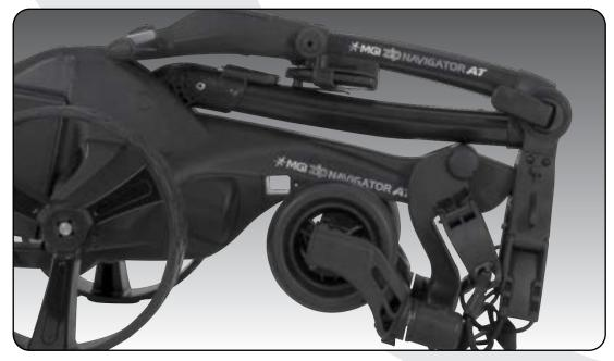
Step 5: Push the toggle down on the top bag support and then move the top bag support down so that it locks over the front wheel assembly.
