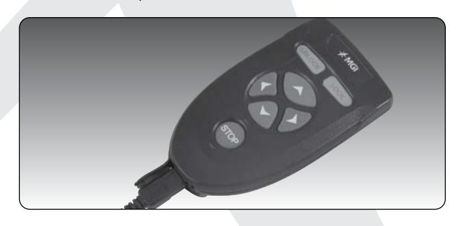
To check the level of power in the remote, press any button to signal the digital top box and the remote control battery level will show on the screen of the Zip Navigator AT.
