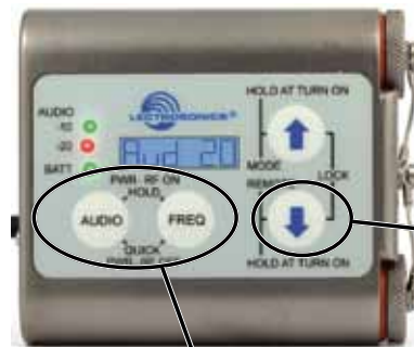
Then press the AUDIO and FREQ buttons at the same time
