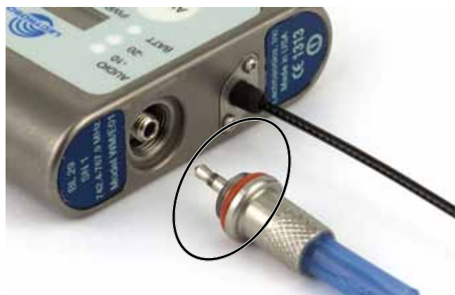
Treat O-ring with petroleum jelly before connecting
