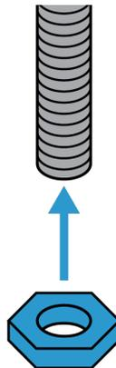
3. Attach the 3/8 in. adapter to the VESA bracket. Thread the VESA bracket onto the threaded rod. Using a wrench, tighten the jam nut against the 3/8 in. adapter.
