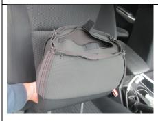
Step 3) Turn the neoprene headrest cover inside out and place on the headrest. **NOTE:** The middle headrest is a slightly smaller headrest
