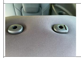
Step 6) Gently place the seat cover over the backrest section. Tuck the holes created in the cover underneath the plastic.
