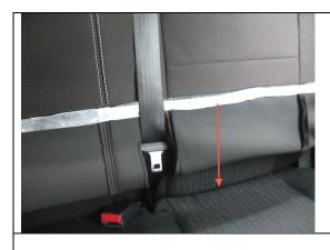
Step 8) Carefully tuck the neoprene between the gap of the cushion and the backrest. This will be used to connect the Velcro on the other side. **Note:** It is much easier to tuck the material through the gap when the cushion section is lowered to a 45 degree angle
