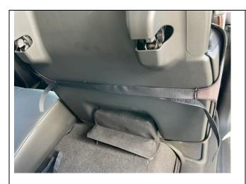
Step 15) Attach the 2 x velcro strips underneath the cushion to secure the cushion section. Ensure that that the Velcro is a nice tight fit. Feel free to trim off a bit of the Velcro, if the straps are too long
