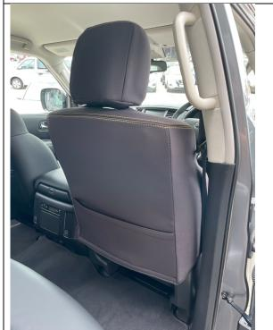
Step 10) We have sewn 3 x Velcro strap directly under the map pocket. Remove the protective touch tape and affix to the carpet underneath the map pocket
