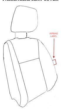
b) When fitting the seat cover over the backrest section – It is very important that you aren't too rough in the fitment (particularly on the 2 airbag panels). You should carefully lower the cover at the same rate. If one side is drastically favoured when fitted, it will stretch the opposing panel, which may potentially tear the seat covers special stitching, which has been designed specifically for airbag safety / deployment. We will discuss this further in the steps below.
