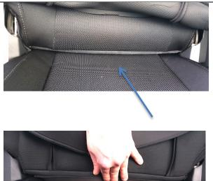
Step 8) Once the backrest section is correctly fitted you can then push the dowel pocket through the gap between the cushion and the backrest. **The first illustration to the left** indicates the gap in which the dowel pocket should be pushed through.
