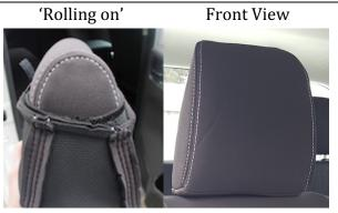
Step 3) Roll the headrest cover onto the headrest (the headrest cover should no longer be inside out). The 'Feature thread' should be facing the front. The back sewn thread facing the rear – As per the photos to the left.
