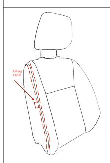
Step 7) Please ensure that our 'Airbag seam' is closely aligned to the original seats 'Airbag seam'. If you need to re-align the seat cover seam in any way, please do so by 'pinching' the 2 panels together and maneuvering the seat cover airbag panels to the correct position. Don't pull the panels across for re-alignment, as this could potentially tear the airbag seam.
