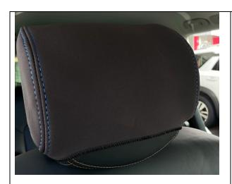
Step 6d) **AN EXAMPLE OF INCORRECT FITMENT** – You must remove the cover and follow Steps 6a to 6c again as you have fitted it the wrong way around.
