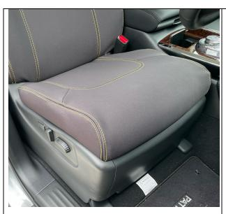
Step 9) Ensure that the excess neoprene on the cushion section is tucked between the gap of the original trim and the plastic (NOT OVER THE TOP OF THE PLASTIC)
