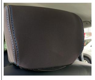
Please Note: There may be a small amount of exposed material at the front of the headrest. There was no real way of overcoming this due to the constraints of the fixed headrest and the method in which we need to sew the panels together. If too much material is showing, you have not fitted the headrest cover correctly. See example below of an incorrect fitment.
