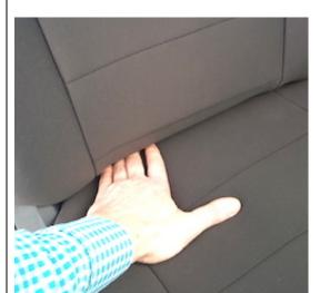
The third illustration to the left showcases a very poorly fitted seat cover. If there is too much 'bunching up' of material it means that you have not tucked enough of the dowel / neoprene through the gap between the cushion and the backrest. Our seat covers have been specially designed so that the seat cover can still be in operation / comfortable when the seats are fully reclined, which is why it is important to tuck the neoprene through the gap, when the seats are in an upright position.
