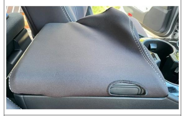
**Step 4)** Once closed on the drivers side, lift the passengers side latch so you can then fit the front passengers side section. And then close.
