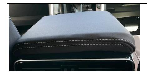
**IF THE CONSOLE COVER IS NOT CLOSING** – Please lift the console and have a look. It's likely that you have pulled down a section too far downwards – either in the corner or on the side which is creating an obstruction on closure.
