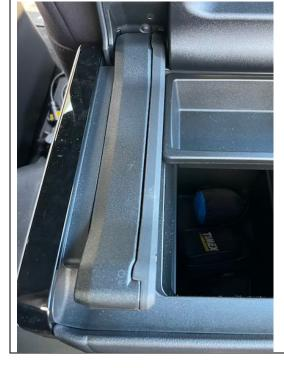
**Step 3)** Fit the 3 corners first. At this stage you won't be able to fit the front passengers side section.
