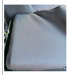
Once all 3 sides have been tucked under correctly lower the console on the drivers side. It may take a little bit of force to flatten it down at this point. **If it won't close** it means you have fitted it incorrectly and the material is interfering. Please lift the console and have a look. It's likely that you have pulled down a section too far downwards – either in the corner or on the side which is creating an obstruction on closure.
