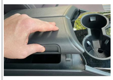
**Step 2)** With the console raised slightly on the drivers side (as per step 1) press the passengers side button and lift the back of the console up.
