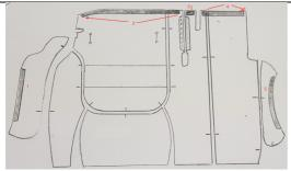
Step 13) Once velcro is affixed in step 12, push the excess neoprene through the gap of the cushion and backrest. This is done easiest by lowering the backrest to a 45 degree angle. Also tuck the neoprene down on the side of the cover. Refer to the diagram to the left of the plastic tab positions on the cover that must be pushed upwards in Step 14. There are 5 in total – 2 on the side and 3 at the back.
