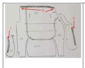
Step 15) **40% Cushion Fitment -** Place cushion cover over the cushion. It only needs to be done roughly at this point in time. Follow steps 11 through to 14. Please Note: Velcro Fitment in Step 12 is not applicable. Refer to the diagram to the left of the plastic tab positions on the cover that must be pushed upwards. There are 3 in total for the 40% Cushion – 2 on the side and 1 at the back.
