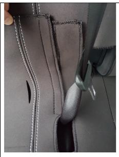
Step 12) Prior to pushing the cover through the gap of the cushion and backrest join velcro together near the middle seat belt (see pic)
