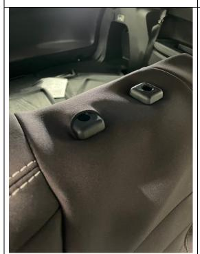
Step 7) Once fitted, ensure that the tag, which is used to lower the backrest, is pulled through the provided hole.
