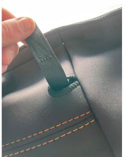
Step 8) The holes that have been created in the seat cover should be tucked under the plastic housing, as per the photos. Start at the front of the plastic and then work your way back.
