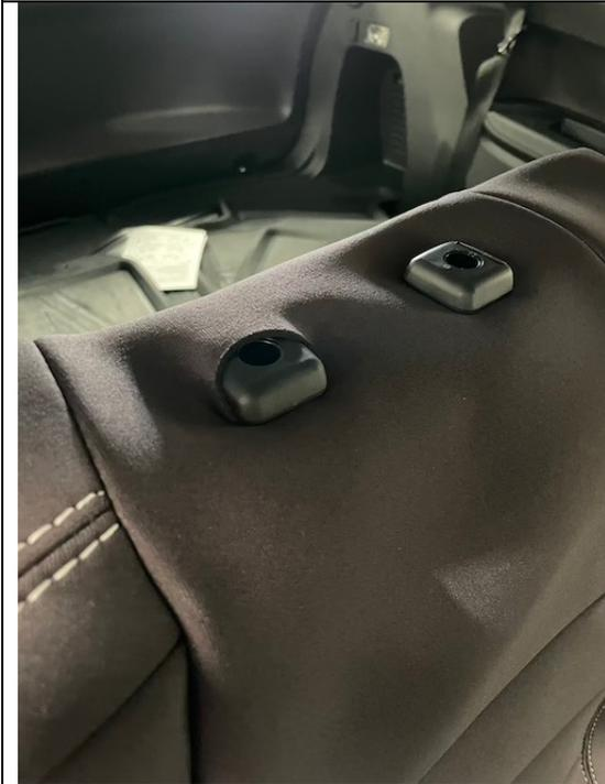
Step 8) The holes that have been created in the seat cover should be tucked under the plastic housing, as per the photos. Start at the front of the plastic and then work your way back.
