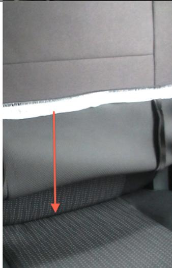
Step 9) Carefully push the neoprene between the gap of the backrest and the cushion. This will be used to join the touch tape on the other side of the backrest (see Step 10). **Please Note:** It is much easier to tuck the material through the gap when the backrest is lowered to a 45 degree angle.
