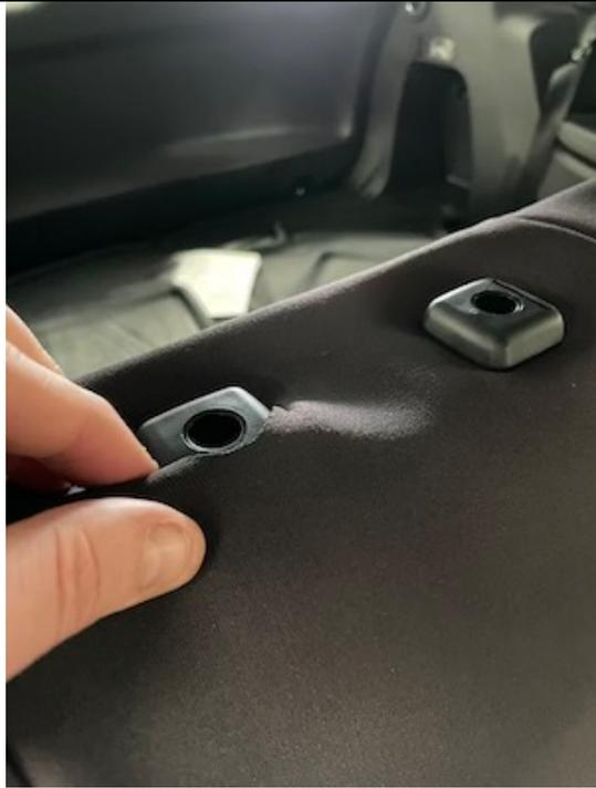
Step 8a) **IF YOU EVER REMOVE THE SEAT COVER**, be careful with the removal, so you don't tear the holes. Start at the front of the seat cover and pinch the seat cover upwards and then work towards the back.
