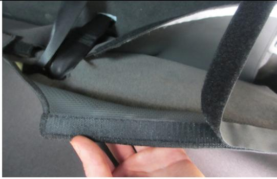
Step 10) Fold the seat flat and remove the protective touch tape. This will allow you to affix the touch tape to the carpet on the back of the seat.
