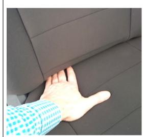
The third illustration to the left showcases a very poorly fitted seat cover. If there is too much 'bunching up' of material it means that you have not tucked enough of the excess neoprene through the gap between the cushion and the backrest. Our seat covers have been specially designed so that the seat cover can still be in operation / comfortable when the seats are fully reclined, which is why it is important to tuck the neoprene through the gap, when the seats are in an upright position.
