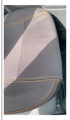
If enough of the excess neoprene is not fed through the gap of the cushion and backrest section it will bunch up at the front, like the below photo. This is an example of a poor fitment.
