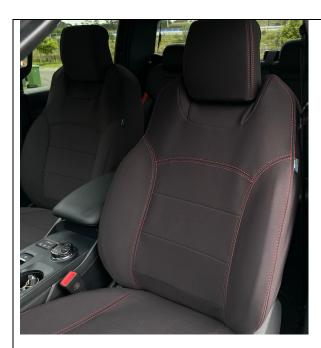
If fitted correctly your seat cover should look like this. The critical element is pushing enough of the excess neoprene and dowel through the gap of the cushion and backrest section.
