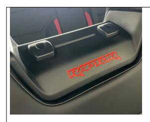
Step 7) Due to the Raptor having plastic underneath the headrest plastic it may not be possible to tuck the headrest underneath like the below photo. It may just need to sit above the headrest plastic (this won't impact fitment in any way)
