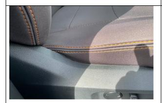
Step 9) **CUSHION FITMENT** – To ensure that the cover is fitted correctly there should be no exposed material showing. The "ears" of the seat cover should also slot nicely into a little gap within the plastic and the original trim.
