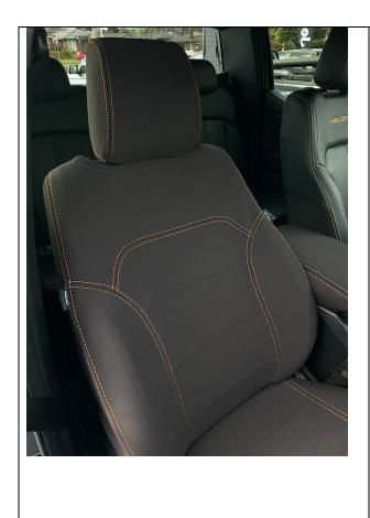
If fitted correctly your seat cover should look like this. The critical element is pushing enough of the excess neoprene and dowel through the gap of the cushion and backrest section.
