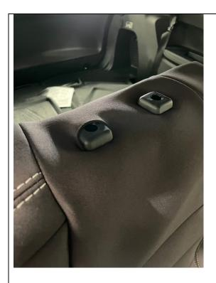
Step 7) The holes that have been created in the seat cover should be tucked under the plastic housing, as per the photos. Start at the front of the plastic and then work your way back.
