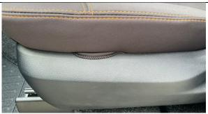
Step 11) There is a small point when fitting the cushion section, in which it becomes very tight to fit (see photo to the left). We suggest, using a small blunt object, such as a ruler to push the neoprene through this gap.
