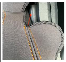
step 10) **CUSHION FITMENT** – To ensure that the cover is fitted correctly there should be no exposed material showing. In the photo to left, more of the excess neoprene needs to be fed through so there is no material showing. The "ears" of the seat cover should also slot nicely into a little gap within the plastic and the original trim.
