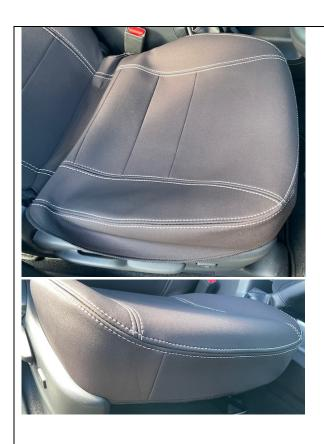
Step 9) **Cushion Fitment** – **CORRECT FITMENT.** Start off by aligning the seat cover at the front of the cushion **(THIS IS A CRITICAL STEP)**. The twin needle stitching should be aligned as per the photos to the left / below, not too low down (like we saw in step 8). When fitted correctly, there will be bunching up of the neoprene towards the backrest section. The excess neoprene will be rectified in Step 10.
