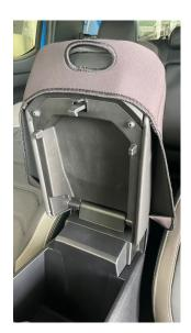
**Step 2)** Tuck the 2 x ears in at the bottom of the console
