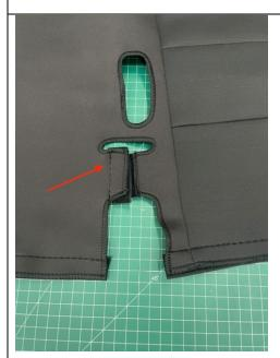
Step 16) We have created a slit in the seat cover to allow the middle seat belt to go through the seat cover. Once the middle seat belt is through the cover (see the photo to the left and below) you can then join the seat cover together – NOTE: you will need to remove the Velcro protective layer first so that it will stick together.
