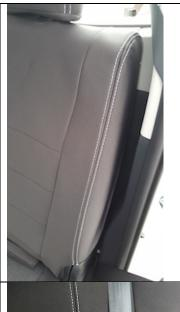
Step 9) Ensure that the shoulders of the seat cover (on both sides) are tucked in nicely. There is a small gap in which the material can also be pushed through.
