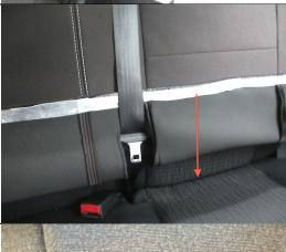
Step 10) Carefully tuck the neoprene between the gap of the backrest and the cushion. **Note:** It is much easier to tuck the material through the gap when the cushion section is raised (Please refer to step 14) to see how you can lift up the cushion)
