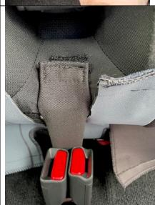
Step 14) It's important to note: that there are 2 x tabs that Nissan have sewn into the cushion section. These cannot be removed (it's to hold the seat belt buckles into place). We have created 2 x cutouts so that the cover can be fitted around these tabs- see below
