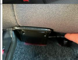
Step 11) There are 4 x isofix points located throughout the seat. To ensure you can still access the isofix points, it's critical that you tuck the cover between the gap of the isofix point and the original seat (as per the left). DON'T GO OVER THE TOP OF THE ISOFIX BAR LIKE THE PHOTO BELOW
