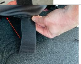
Step 13) Attach the Velcro to the carpet on the floor. Attach towards the back of the vehicle, as this will create more tension on the seat cover and make it a tighter fit. Be careful not to be too tight as it might tear the seat cover.
