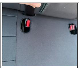
Step 15) After the cushion is raised, place the cover over the cushion. Tuck the neoprene through the gap between the cushion and the backrest. Prior to removing the protective touch tape (step 17), ensure that you are happy with the fitment. Ensure that the holes in the seat cover cushion are aligned with the seat belt buckles
