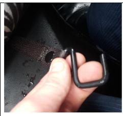
Step 9) – To raise the cushion section simply pull the strap and then lift the cushion section.
