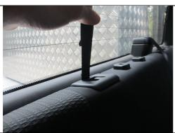
Step 6) **Backrest Fitment** – Lower the backrest by pulling the tag on the top left and right hand side. For the easiest fitment of the backrest seat cover, lower the backrest to a 45-degree angle.
