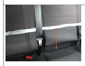
Step 8) Carefully tuck the neoprene between the gap of the backrest and the cushion. This will be used to join the velcro to the carpet on the other side of the backrest. **Note:** It is much easier to tuck the material through the gap when the cushion section is lifted up (Please refer to step 9 to see how you can lift up the cushion)
