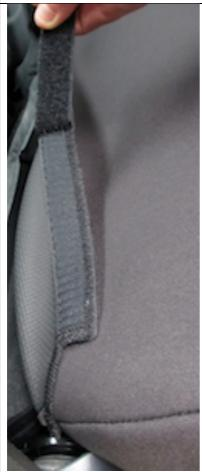
Step 10) In this step you will fit the velcro to the carpet, which is located on the back of the backrest.
