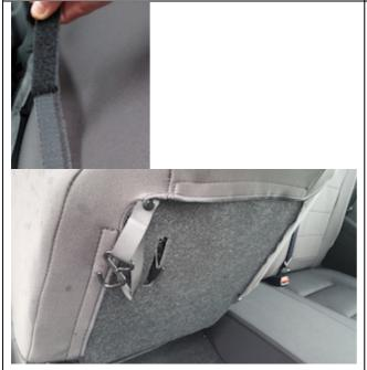
Step 13) If happy with the fitment in Step 12, lift the cushion section up and remove the protective touch tape. Affix the velcro to the carpet on the cushion section, as per the photos to the left.
