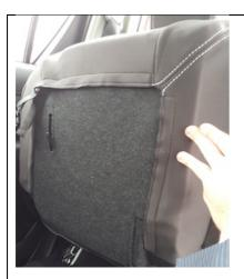
Step 12) After the cushion is raised, place the appropriate cover over the cushion. Tuck the neoprene through the gap between the cushion and the backrest. Prior to removing the protective touch tape, ensure that you are happy with the fitment. See the photo below of how the cushion should be fitted (The photo to the left is of the Toyota Hilux rear – however the same principles apply)
