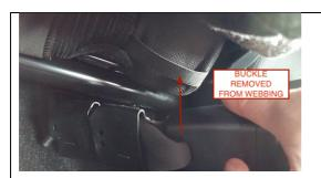
Step 5) Prior to the upcoming steps it is important to remove the seat belt buckles from their webbing. To do this simply lift up the cushion (Refer to step 9 to see how you can lift up the cushion) and remove the buckles from their webbing and place on the floor.
