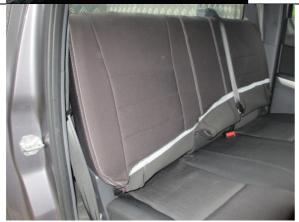
Step 7) Place the backrest cover over the seat back. To ensure the easiest possible fitment, you should re-fit one headrest at a time through the eyelets. This will act as a locking mechanism for the seat cover, so that it can be fitted much easier in the later steps. **Note:** Ensure that the cover is fitted underneath the seat belt (not over the top of it). Once fitted, ensure that the tags, which are used to lower the backrest, are lined up and gently pulled through the slits.
