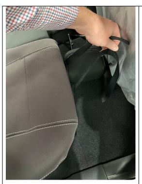
Step 10) **40% Cushion Fitment** –Start off by aligning the seat cover at the front of the cushion. Please ensuring that the Velcro at the front is brought outwards prior to fitting (see pic)
