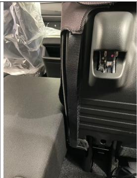
Step 13) Join the long Velcro strip that is located closest to the centre of the vehicle.
