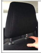
Step 2) Remove all headrests by pressing the button on the right hand side and lifting the headrest until it cannot be raised any further.
