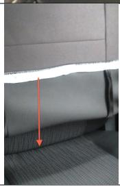
Step 7) Carefully push the neoprene between the gap of the backrest and the cushion. This will be used to join the touch tape on the other side of the backrest (see Step 8). **Please Note:** It is much easier to tuck the material through the gap when the backrest is lowered to a 45 degree angle.
