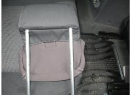
Step 3a) As per the pictures to the left and below, fit the headrest cover by placing the headrest into the headrest cover. Squeeze the foam in the headrest to make it easier to fit the headrest cover. **Note:** Please be gentle when fitting the headrest cover, as it is a tight, custom-fit design. THE PHOTOS ARE ILLUSTRATIONS ONLY AND MAY NOT BE THE SAME HEADRESTS COVERS
