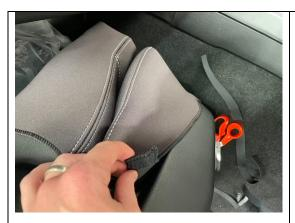
Step 15) Slot other small velcro (door side) in between the gap. It then affixes to carpet, internally. You'll need to remove protective touch tape layer prior to fitting section.
