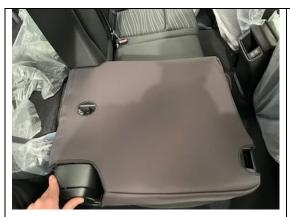
Step 8) Fold the seat flat and join the 2 velcro tabs together that are located on the back of the cover. (as per the picture to the left). Note: You will need to remove the protective touch tape first from one side (see below).
