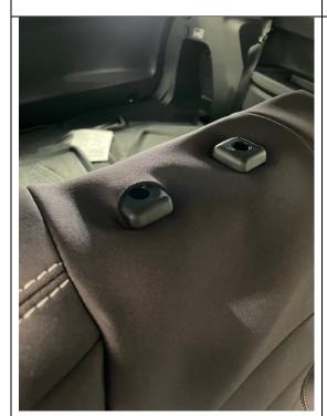
Step 6) The seat cover in the 2<sup>nd</sup> row does not have eyelets inserted into the product. The holes that have been created in the seat cover should be tucked under the plastic housing, as per the photos. Start at the front of the plastic and then work your way back.
