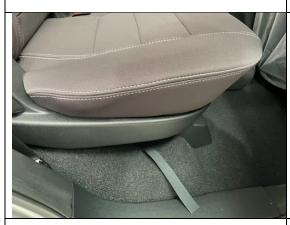
Step 16) Tuck neoprene into the plastic on the side of the seat. To avoid bunching at the front of the seat cover, pinch quite a bit of material at the back and push through as much as possible towards the back of the vehicle. If done incorrectly, there can be a lot of bunching at the front.
