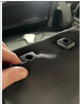
Step 6a) **IF YOU EVER REMOVE THE SEAT COVER**, be careful with the removal, so you don't tear the holes. Start at the front of the seat cover and pinch the seat cover upwards and then work towards the back.
