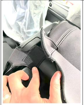
Step 12) Join the 2 x large velcro tabs – These are located closest to the centre of the vehicle.
