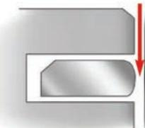
**THE FACE OF THE RING** – The face of any compression ring can have many characteristics that may help or hinder cylinder sealing. The profile (barrel, taper..etc) can vary in many different ways that help the ring stay seated through piston rock over. Face coatings can also make a substantial difference with cylinder sealing depending on your cylinder wall material.
