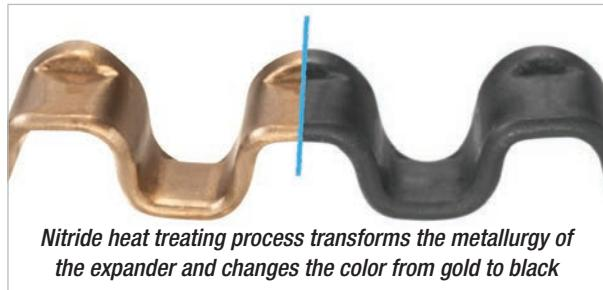
*Nitride heat treating process transforms the metallurgy of the expander and changes the color from gold to black*
