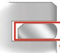
**THE SIDES OF THE RING** – The side surfaces of the ring, that is the surfaces that seat against the piston flank itself are often overlooked but equally as important in sealing an engine. Simply, the flatter and smoother these sides are, the better they will seal against the piston and stop any blow-by from traveling around the ring land and into the crankcase.
