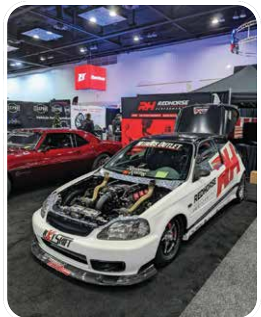
Thomas West's RWD nitrous injected, twin turbo, stick shift 427ci LS swapped Honda Civic #RhPlumbed
