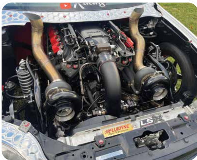
Thomas West's RWD nitrous injected, twin turbo, stick shift 427ci LS swapped Honda Civic #RhPlumbed
