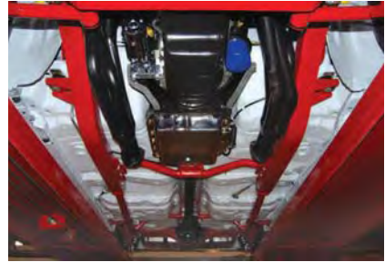
4. HEIDTS® Front Subframe with Subframe Connectors joins to HEIDTS® Rear 4-Link Kit.
