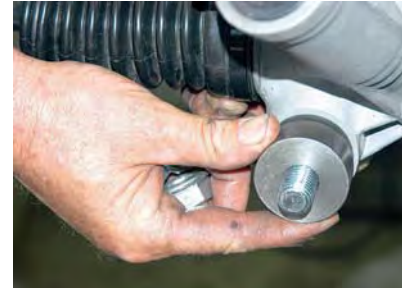
25) Before the rack-and-pinion can be installed, you have to install the bolts with a pair of spacers and washers.
