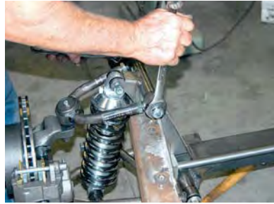
23) After all the front suspension parts are installed, the bolts can be tightened. The upper A-arm bolts were secured with a pair of 15/16-inch wrenches.
