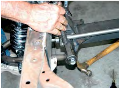
24) The lower A-arm bolt and Nylok locknut was secured with a pair of 15/16-inch wrenches.
