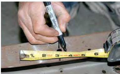
4 According to the instructions, the centerline for the HEIDTS® suspension will be 1/2 inch back from the straight-axle centerline.
