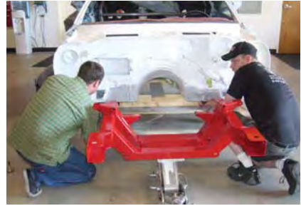
2. The new HEIDTS® Front Subframe and only four bolts, completes the installation to the body.
