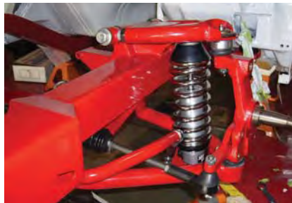
3. HEIDTS® 2” Drop Spindle and Upper and Lower Arms mount to HEIDTS® subframe.
