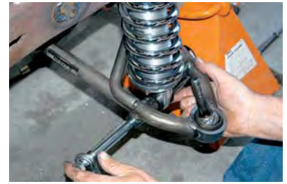
16) The coilover shock was connected to the lower A-arm. This is a long bolt because it is also used to secure the Swaybar connector. The bolt is installed from the front and O'Bryant made sure the Swaybar connector was installed first.
