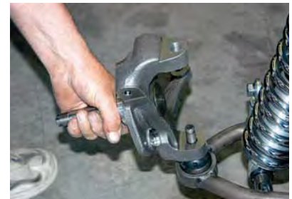
17) The spindle was connected to the lower A-arm. The lower ball joint is long, so spacers are used to make sure the castle nut aligns with the cotter keyhole.
