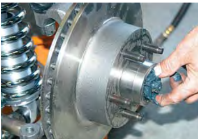
21) The rotor was installed on the spindle and then the small spindle bearing was installed. It was also packed with high-heat disc-brake bearing grease.
