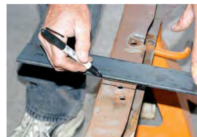
5) The HEIDTS® centerline was drawn on top of the frame to make it easy to spot.
