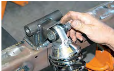
14) Bolting the coilover shock to the upper tower started the installation. At this point the bolt was finger-tight just in case it would have to be removed.
