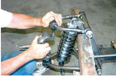
19) Now the upper A-arm can be connected to the spindle. HEIDTS® recommended using one of its narrow front suspension kits to keep the tires inside the fenderwell so the tires don't hit on turns.
