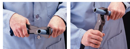
The rotating/rocking technique produces fast easy cuts.
