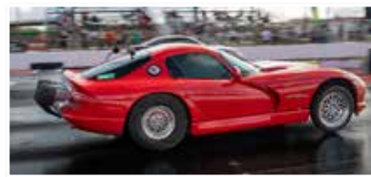
"THE JUGGERNAUT" VIPER 6.89 @205 mph World's Quickest IRS Gen II Viper built by Nth Moto Gen II Viper with Gen V Engine Combo ATI Max Duty Outlaw Lock Up T400 Transmission, Torque Converter, Super Damper
