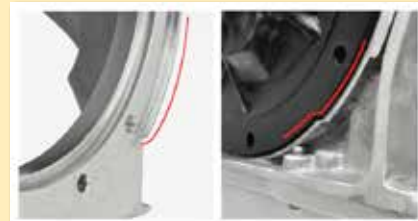
ATI custom machines an indicating guide into the OEM case to accept a new SFI Direct Fit Bell for a perfect fit.
