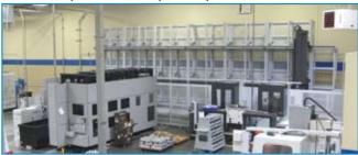
2 Mori Seiki Twin Pallet CNC Machines Feeding a 42 Pallet Shuttle Cell
