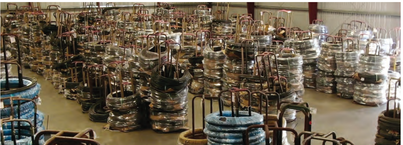
Material comes from the mill in large coils...which subsequently will be fed into cold-headers and formed into bolts.
