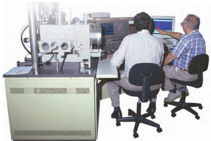
ARP engineers use "Scanning Electron Microscopic" inspection capable of detecting all elements in the periodic table with atomic numbers greater than 5 – permitting the acquisition of high resolution imaging.
