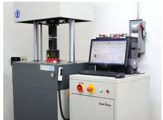
ARP has two highly sophisticated Amsler fatigue machines, which test fasteners through millions of cycles.
