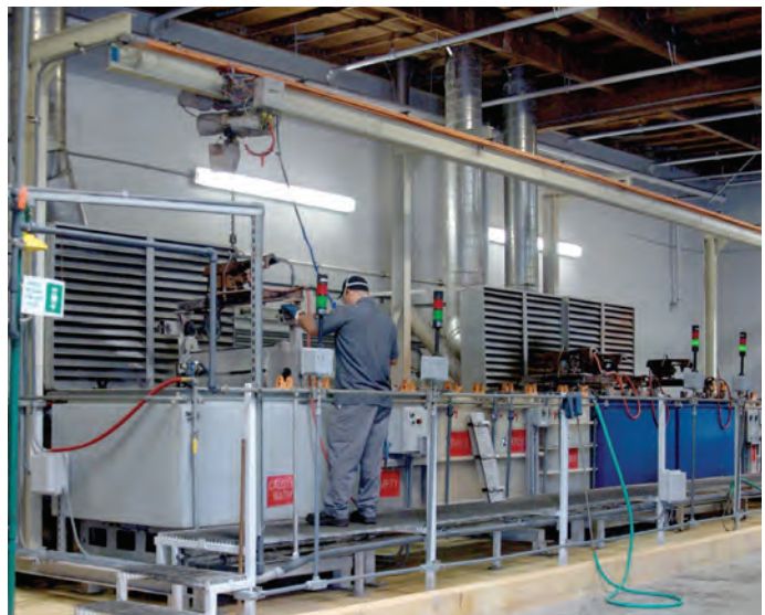
The finishing touch for most chrome moly fasteners is the black oxidizing operation.
