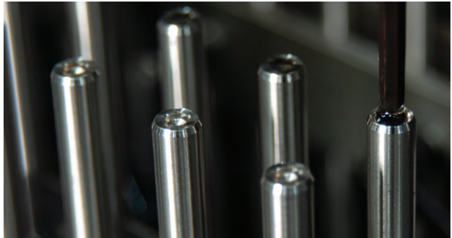
State-of-the-art EDM technology is used to perform special operations, such as hex-broaching head studs.
