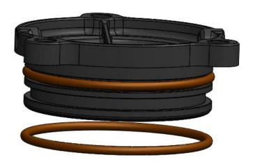
2. Press the filter cover straight into the oil filter bore. Tighten the (3x) M6 screws to 10 Nm (7.38 ft-lb) with an 8 mm socket and torque wrench.
