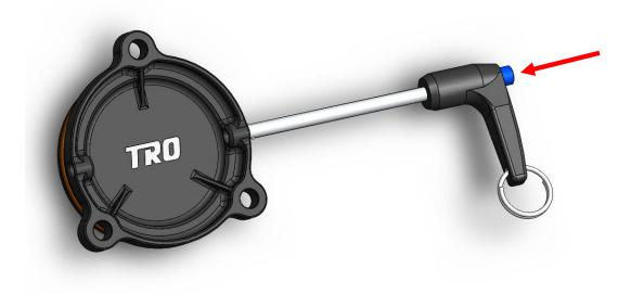
3. Using pliers or vice grips, grip the pin from the center of the filter cover and pull the cover out of the engine. For extra stability during removal, use one hand to guide the filter cover and one hand to remove it with pliers.
