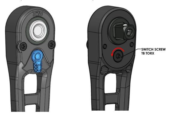
2. Remove both cover plate screws using a T10 Torx L-key.
