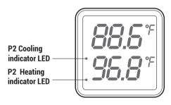
**P2 Heating indicator LED:** If P2 Temperature Control Function selected heating mode, the indicator LED is on, otherwise off.
