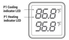
**P1 Heating indicator LED:** If P1 Temperature Control Function selected heating mode, the indicator LED is on, otherwise off.
