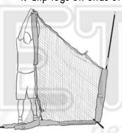
Slip loop over the rod top, repeat on other pole by pulling orange sleeve up and loop cord over pole
