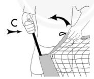
Grip Rod pushing direction (C) whilst pulling Orange sleeve up and looping Cord over Poll Top
