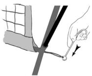
10. Stake thru ring into ground applying a little tension to bungee. Repeat on other side
