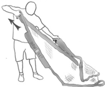
1. Holding both Tubes, pull one side of Net Frame out until it locks (click sound)
