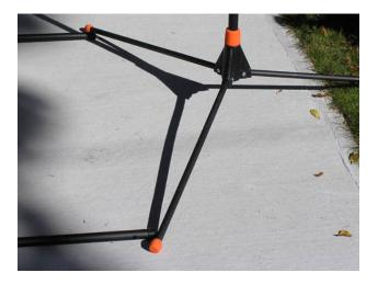
1. The tripod for the electronic display module must be positioned with two of its legs just behind the back legs of the pitching screen. This assures the correct location for proper operation and protection of the electronic module
