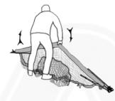
Swing net open and place one hinge on the ground then open to full width, and lay both hinges on the ground
