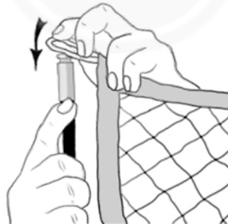
8. Grip Black Rod pulling Orange sleeve up and loop Cord over Poll Top
