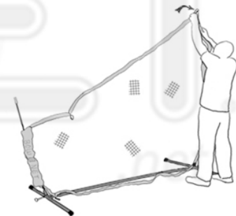
6. Hold Black Rod pulling Orange sleeve up and loop White Cord over rod top See #8.
