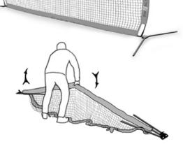
3. Open to full width, laying both hinges on the ground.
