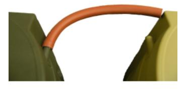
**4)** Slide metal clamps onto tube and connect other end to drilled node on other barrel
