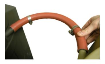
**5)** Slide clamps towards end of hose and strongly tighten using flat head screw driver
